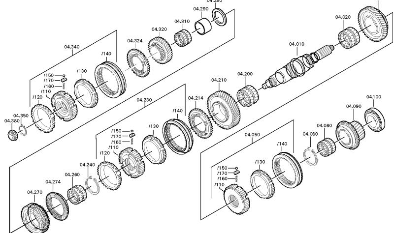
Plant Page 2 from 2 Material number: 1307.050.366 Plant: 067.04.82-1 MAIN SHAFT S 5-42 / KAMAZ PUBLIC JOINT STOCK COMPANY MAIN SHAFT
