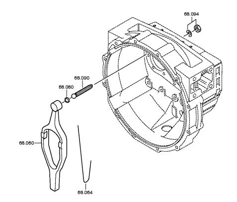
Plant Page 2 from 2 Material number: 1307.050.366 Plant: 067.93.69-1 CLUTCH RELEASE DEVICE S 5-42 / KAMAZ PUBLIC JOINT STOCK COMPANY CLUTCH RELEASE DEVICE
