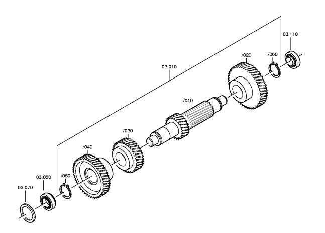
S 5-42 / KAMAZ PUBLIC JOINT STOCK COMPANY Plant Material number: 1307.050.366 Plant: 067.04.04-1 MAIN SHAFT Page 1 from 2 MAIN SHAFT 04.030 04.280
