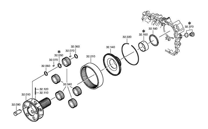
Plant Page 2 from 2 Material number: 1341.002.021 Plant: 068.44.47-1 PLANETARY DRIVE 16 S 1820 TO / RENAULT TRUCKS PLANETARY DRIVE
