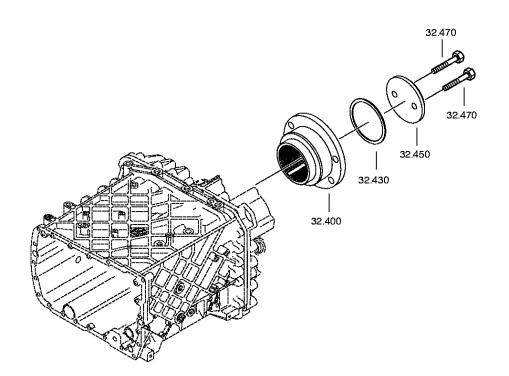
Plant Page 1 from 2 Material number: 1341.002.021 Plant: 068.45.04-1 SYNCHRONIZER 16 S 1820 TO / RENAULT TRUCKS SYNCHRONIZER
