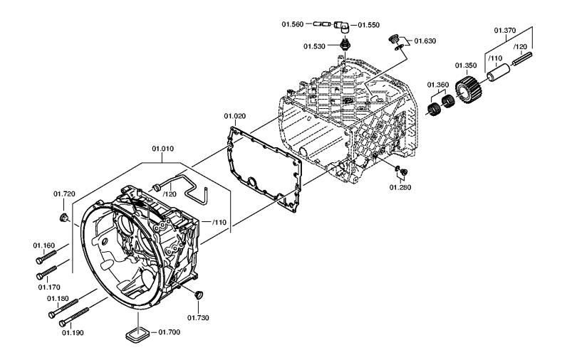
Plant Page 1 from 3 Material number: 1341.002.021 Plant: 068.02.55-1 INPUT SHAFT 16 S 1820 TO / RENAULT TRUCKS CONNPLATE
