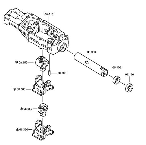
Plant Page 4 from 4 Material number: 1341.002.021 Plant: 068.07.82-1 GEAR SHIFT SHAFT 16 S 1820 TO / RENAULT TRUCKS GEAR SHIFT HOUSING
