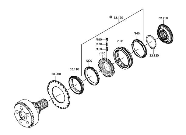
Plant Page 2 from 2 Material number: 1341.002.021 Plant: 068.45.40-1 SYNCHRONIZER 16 S 1820 TO / RENAULT TRUCKS SYNCHRONIZER
