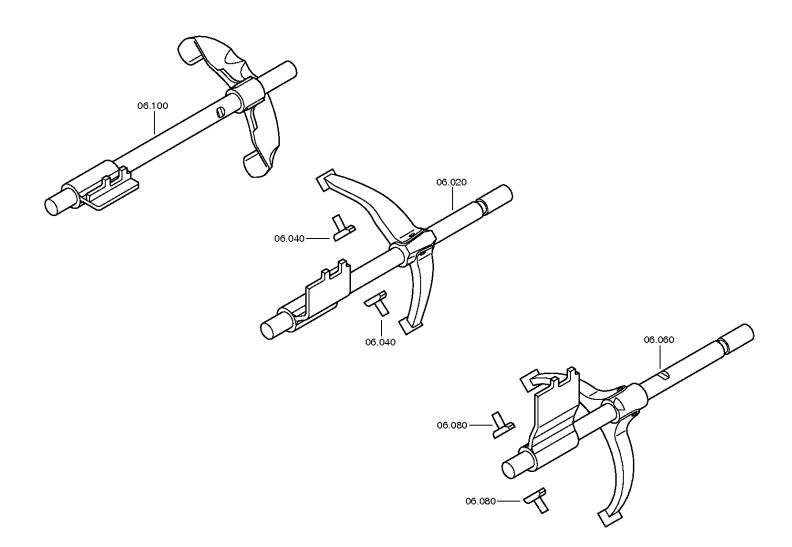
Plant Page 2 from 3 Material number: 1341.002.021 Plant: 068.06.43-1 GEAR SHIFT SYSTEM 16 S 1820 TO / RENAULT TRUCKS GEAR SHIFT SYSTEM
