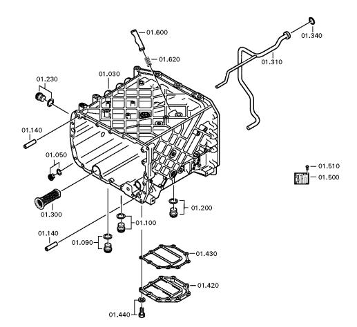
Plant Page 2 from 2 Material number: 1341.002.021 Plant: 068.01.52-1 GEARBOX HOUSING 16 S 1820 TO / RENAULT TRUCKS GEARBOX HOUSING
