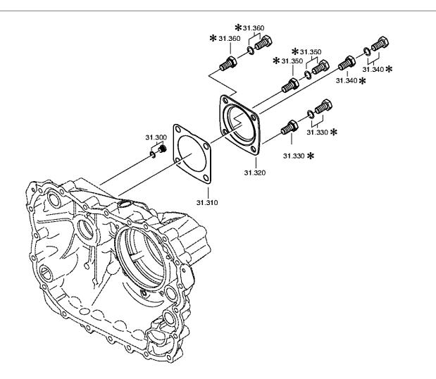
Plant Page 1 from 2 Material number: 1367.002.030 Plant: 161.44.01-1 PLANETARY DRIVE 16 S 2220 TO / IVECO PLANETARY DRIVE
