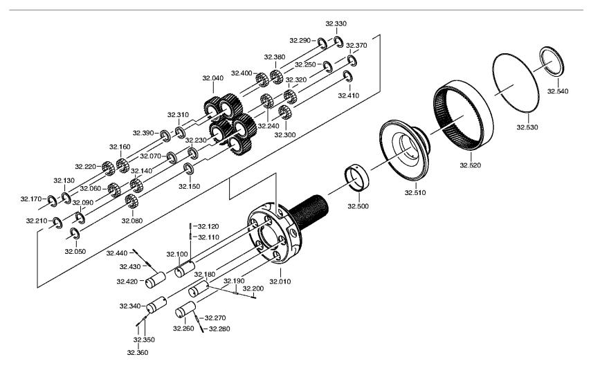
Plant Page 2 from 2 Material number: 1367.002.030 Plant: 161.44.40-1 PLANETARY DRIVE 16 S 2220 TO / IVECO PLANETARY DRIVE
