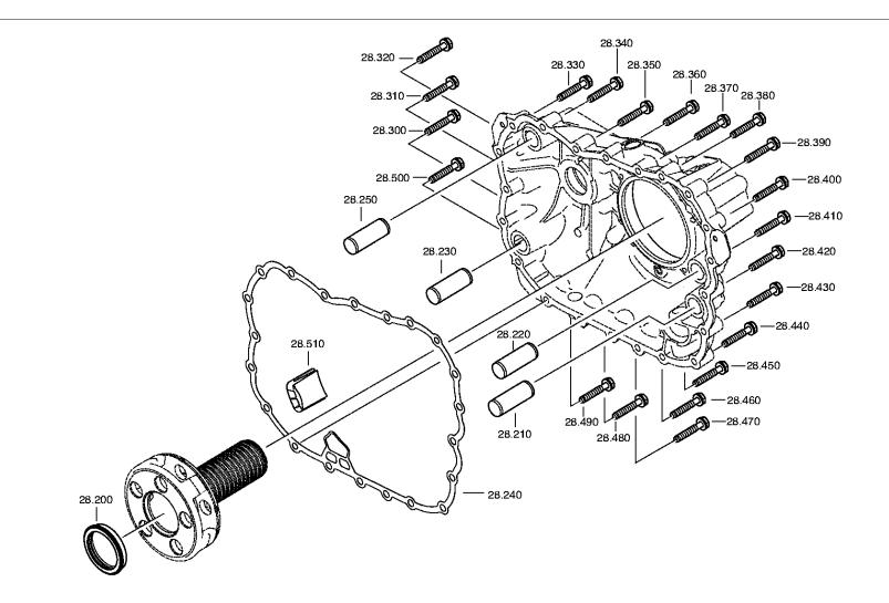
Plant Page 1 from 2 Material number: 1367.002.030 Plant: 161.40.01-1 GV-SHIFT SYSTEM 16 S 2220 TO / IVECO GV-SHIFT SYSTEM
