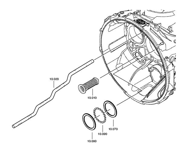
Plant Page 2 from 2 Material number: 1367.002.030 Plant: 161.10.01-1 PUMP 16 S 2220 TO / IVECO OIL SUPLY
