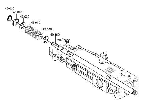
Plant Page 1 from 1 Material number: 1367.002.03016 S 2220 TO / IVECOPlant: 161.28.02-1PLANETARY RANGEMaterial-assembly-group-no: 1367.128.803
